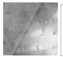
The micrograph on the left (from a transmission electron microscope) represents the plan view of a slip plane with segments of cross-slipped dislocations bowing out from a force being applied to them.
